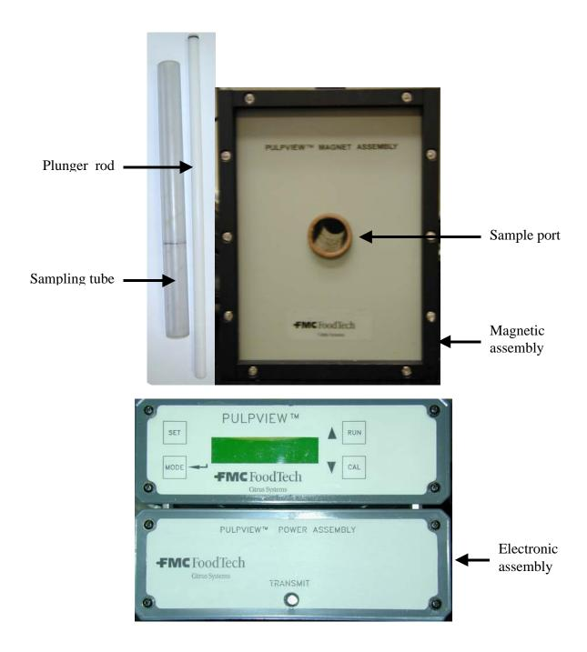
Figure V-1. Magnetic assembly and instrument panels of the FMC FoodTech PulpView<sup>TM</sup>.
