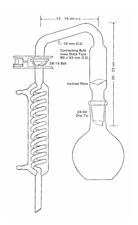
Figure IV - 10. Distillation apparatus used for Scott oil test.
