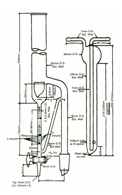
Figure IV-11. Oil separatory trap used for Clevenger method (source: USDA Citrus Handbook).
